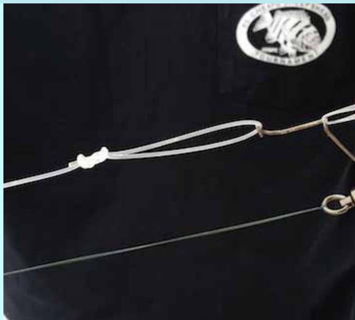
Look closely at this Photo. That is a bent, OPEN snap Swivel that caught a really BIG fish and they landed it like that!
